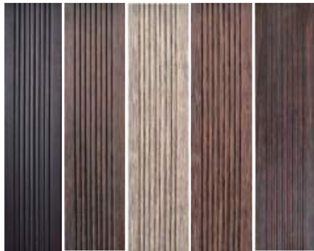
New 6 Months 18 Months After Cleaning After Maintenance
